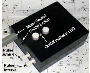
**On/off:** Push slide switch to left to turn on (indicator LED will light), right to turn.
